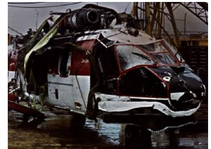
Figure 14: Showing the recovered helicopter onboard MSV Stadive without its main rotor head and main gearbox assembly which detached during the first associated lift from the seabed and was recovered before the main airframe structure shown here.
